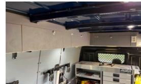
(e) Overhead lockers for storage of equipment
