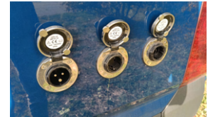
(f) Outlets for power and cable feed-through
